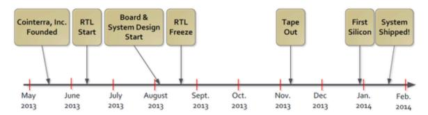
The timeline above shows an example of Bitcoin mining hardware advancing from registertransfer level (RTL) design to 'tapeout', the point at which the graphic for the <u>photomask</u> of the circuit is sent to the fabrication facility in just four months. Normally this takes years.
