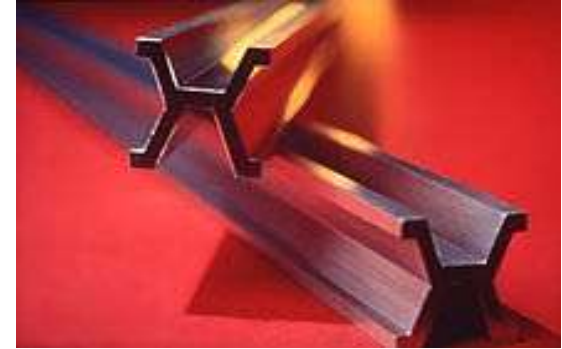
Historical International Prototype Metre bar, made of an alloy of platinum and iridium, that was the standard from 1889 to 1960
